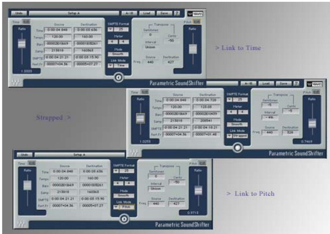
Note that in the Time or Pitch Link modes, the interface will show an arrow pointing to the section that is now dominating the process. The controls of the other section are disabled and therefore appear faded and the Ratio disappears. The disabled section will store whatever settings are there and these settings will get back into action when the link mode is changed.
