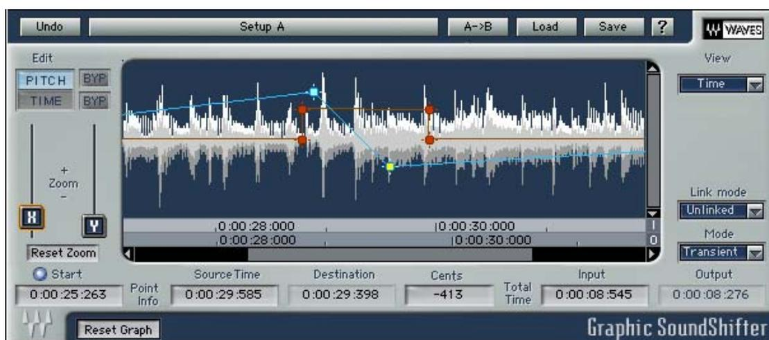
The Graphic SoundShifter takes the very same elements and allows you to program a value change graph across the selection. This is achieved by creating “Points” in the graph that you can drag around to designated timing in the selection at the X axis and to its shift ratio at the Y axis. There are two separate graphs, one for Pitch and one for Time. You can select which one you are editing.
